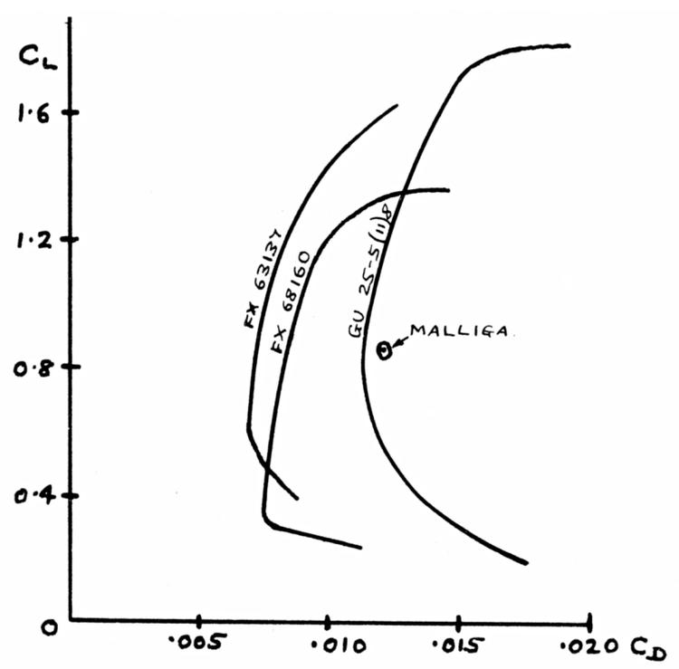
Figure 3. Lift/Drage characteristics.
