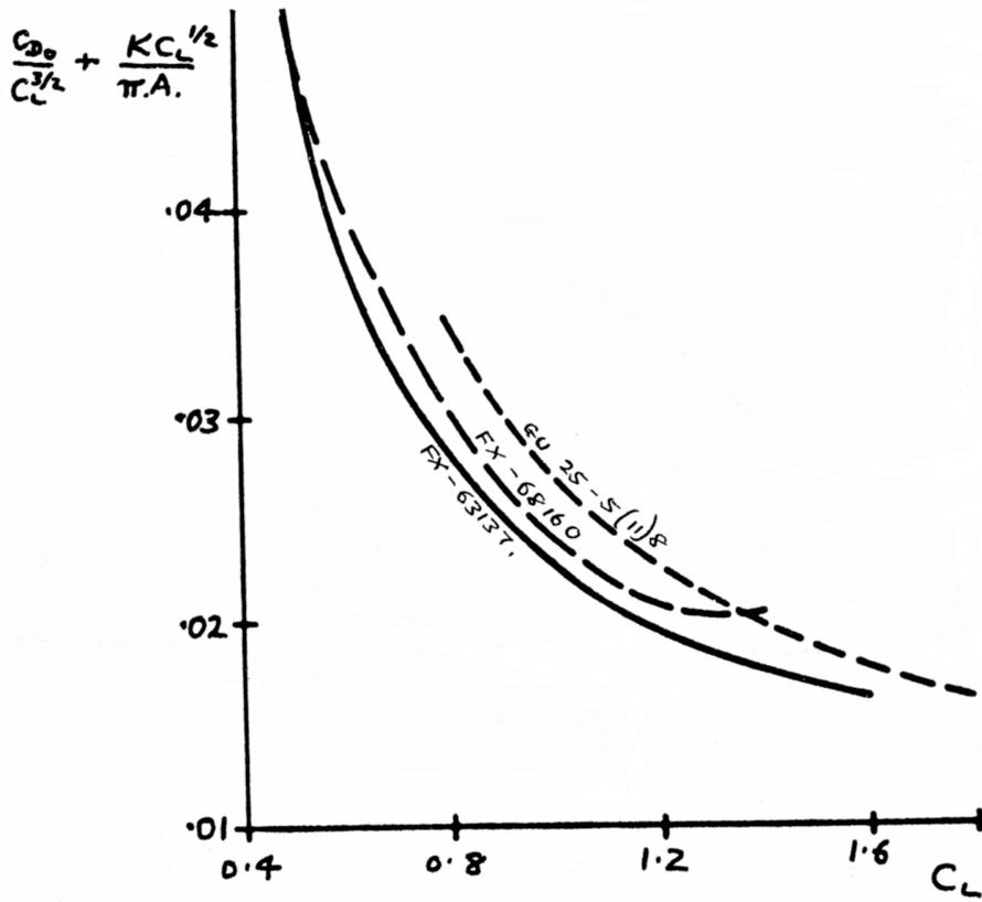
Figure 4. Variation of weight/power parameter with  $C_L$ .
