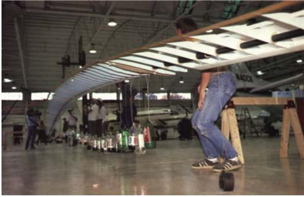
Load testing the Michelob Light Eagle wing using bottles filled with water.
