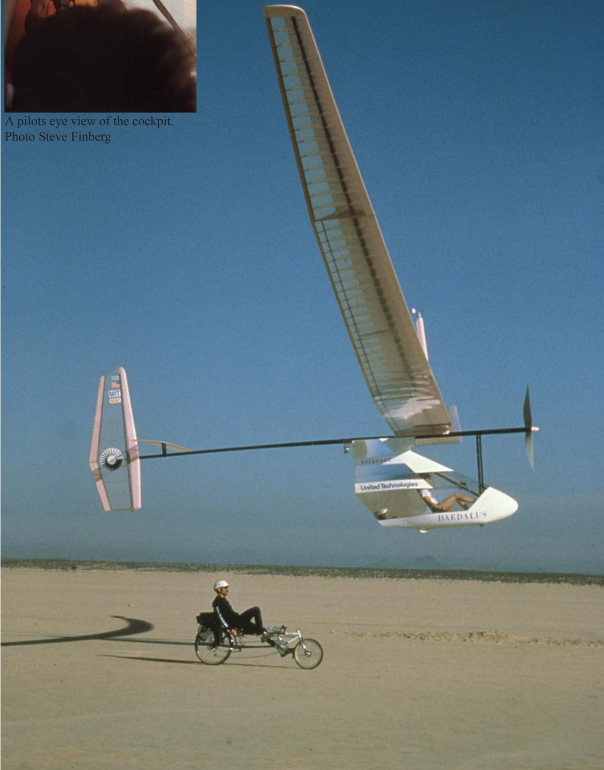
Ryan recumbent cycle paces Daedalus 'A' over the vast flats of Edwards air force base in California. Significantly, with experienced cyclists the aerodynamic efficiency of the human powered aircraft enables aircrew drive to match the effort required for the wheeled bicycle. Photo Steve Finberg
