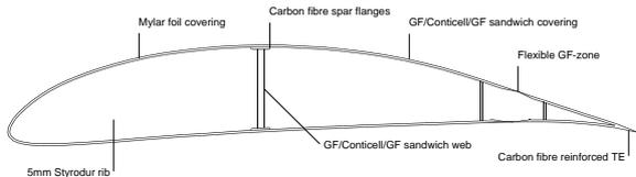
Fig 7. Wing structure of Musculair 2 Wortman airfoil FX 76 A, modified by D. Althaus.
