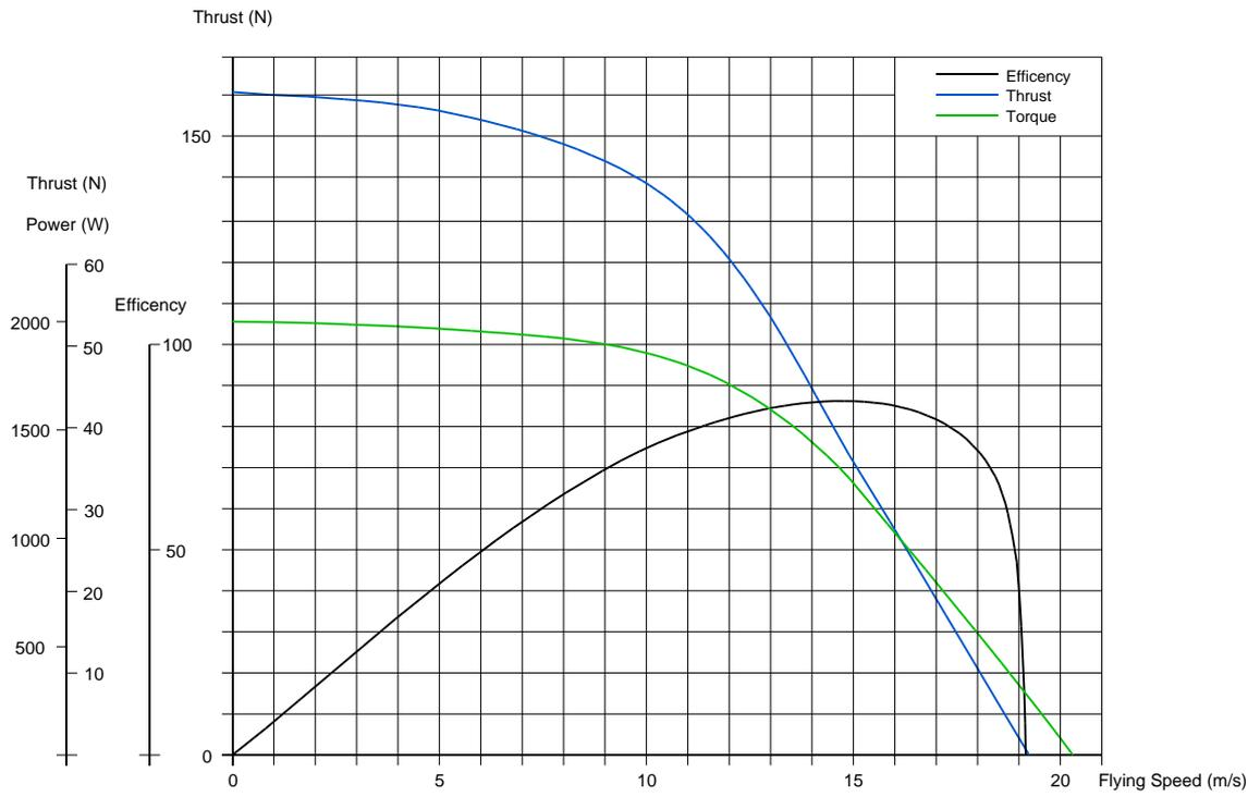
Fig 9 Propeller operation graphs at 360 rpm (wind tunnel test)
