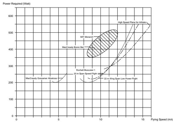
Fig. 2: Power Requirement of Man powered Planes
