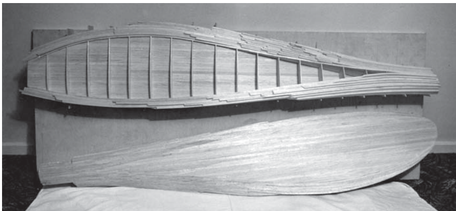
Propeller, balsa laminated outline, ribs and sheeting
