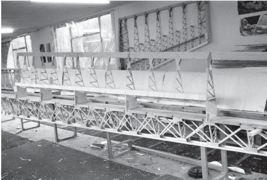
Braced box inverted, aileron slot sub-assembly, TE and ribs
