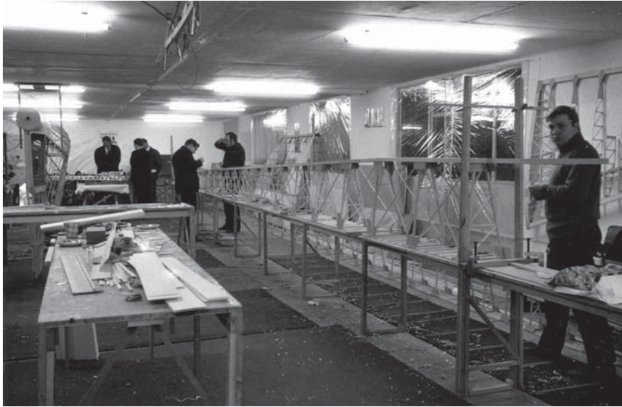
Wing assembly, spruce and ply spar, balsa nose spar and ribs
